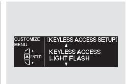
While the multi-information display is in the KEYLESS ACCESS SETUP screen of the CUSTOMIZE GROUP, press the SEL/RESET button. The screen changes to CUSTOMIZE MENU. Press the INFO (▲/▼) button until you see the above display.
