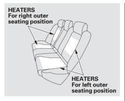
The outer rear seat cushions and seat-backs are equipped with seat heaters.
