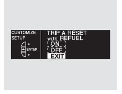
To exit TRIP A RESET with REFUEL without changing the current setting, select EXIT by pressing the INFO (▲/▼) button, then press the SEL/RESET button. The screen goes back to CUSTOMIZE MENU.
