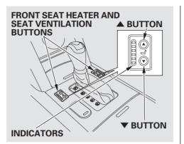
The ignition switch must be in the ON (II) position to use the heaters and the air ventilation system.
