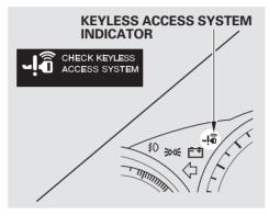
The indicator comes on for several seconds when you turn the ignition switch to the ON (II) position. Have your vehicle checked by your dealer if:
