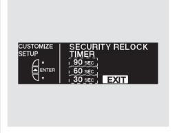
To exit SECURITY RELOCK TIMER without changing the current setting, select EXIT by pressing the INFO (▲/▼) button, then press the SEL/RESET button. The screen goes back to CUSTOMIZE MENU.
