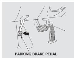
To apply the parking brake, push the parking brake pedal down with your foot. To release the parking brake, push on the pedal again. The parking brake indicator on the instrument panel should go out when the parking brake is fully released with the engine running (see page 63).
