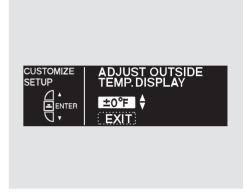
Press the SEL/RESET button. The screen changes as shown above. The highlighted number is the current setting above or below the outside temperature. Press the INFO (▲/▼) button repeatedly until the number you want appears, then press the SEL/RESET button to enter your selection.
