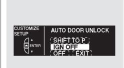
Press the SEL/RESET button. The screen changes as shown above. Select the desired setting by pressing the INFO (▲/▼) button, then press the SEL/RESET button to enter your selection.
