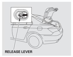
As a safety feature, your vehicle has a release lever on the right corner in the trunk so the trunk can be opened from the inside. To open the trunk, push the release lever in the direction indicated by the arrow.
