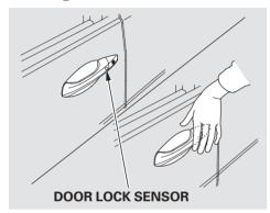
Each front door has a LOCK/UNLOCK feature.
