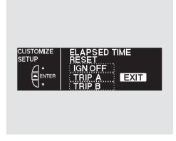
To exit ELAPSED TIME RESET without changing the current setting, select EXIT by pressing the INFO (▲/▼) button, then press the SEL/RESET button. The screen goes back to CUSTOMIZE MENU.
