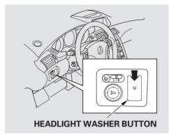
The headlight washers can be operated at any time by pressing the headlight washer button located next to the steering wheel column. The headlights must be turned on to use this button. In addition, the headlight washer operates without pressing the button at the first time you turn on the windshield washers after you turn the ignition switch to the ON (II) position.
