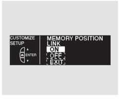
Press the SEL/RESET button. The screen changes as shown above. Select ON or OFF by pressing the INFO (▲/▼) button, then press the SEL/RESET button to enter your selection.
