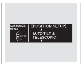
While the multi-information display is in the POSITION SETUP screen of the CUSTOMIZE GROUP, press the SEL/RESET button. The screen changes to CUSTOMIZE MENU. Press the INFO (▲/▼) button until you see the above display.
