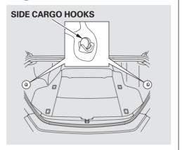
There are hooks on the floor and both sides of the trunk. They can be used to install the cargo net for securing items. The side cargo hooks are designed to hold light items (maximum load: 6 lbs or 3 kgs for each hook). Heavy objects may damage the side hooks.
