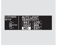
Press the SEL/RESET button. The screen changes as shown above. Select from five levels of sensitivity by pressing the INFO ( $\triangle/\nabla$ ) button, then press the SEL/RESET button to enter your selection.
