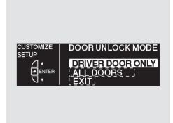
Press the SEL/RESET button. The screen changes as shown above. Select DRIVER DOOR ONLY or ALL DOORS by pressing the INFO (▲/▼) button, then press the SEL/RESET button to enter your selection.
