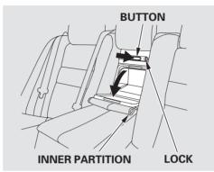
To open the cover, pull down the rear seat armrest. Pull on the tab at the top of the inner partition, and press on the button to fully release the cover. To close the cover, swing it up, and push firmly on the top. Make sure it latches properly.
