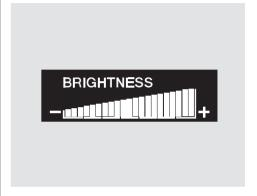
The level of brightness is shown on the multi-information display while you adjust it. It goes out 5 seconds after you finish adjusting.
