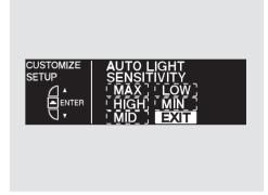
To exit AUTO LIGHT SENSITIVITY without changing the current setting, select EXIT by pressing the INFO (▲/▼) button, then press the SEL/RESET button. The screen goes back to CUSTOMIZE MENU.
