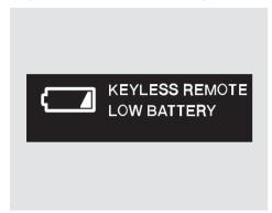
The batteries in the remote normally last about 2 years. To ensure maximum battery life, do not store the remote close to electrical devices such as computers or TVs. When the multi-information display shows "KEYLESS REMOTE LOW BATTERY," replace the batteries as soon as possible (see page 175).
