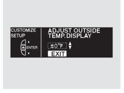
To exit ADJUST OUTSIDE TEMP. DISPLAY without changing the current setting, select EXIT by pressing the INFO (▲/▼) button, then press the SEL/RESET button. The screen goes back to CUSTOMIZE MENU.
