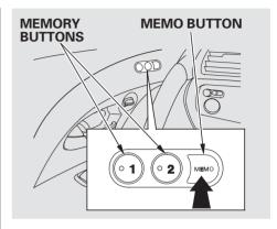
3. Press the MEMO button on the driver's door. You will hear a beep. The indicator in the memory buttons (1 and 2) will blink. Immediately press one of the memory buttons (1 or 2) until you hear two beeps. The indicator in the memory button will stay on. The current positions of the driver's seat, steering wheel, and outside mirrors are now stored.
