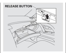
Your vehicle has an owner's manual tray inside the glove box. To open the tray, push the release button up.
