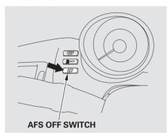
This switch is at the right side of the left vent. Press it to turn the AFS on and off. When AFS is off, the AFS indicator comes on as a reminder when you turn on the headlights.
