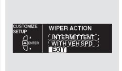
To exit WIPER ACTION without changing the current setting, select EXIT by pressing the INFO (▲/▼) button, then press the SEL/RESET button. The screen goes back to CUSTOMIZE MENU.
