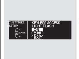
Press the SEL/RESET button. The screen changes as shown above. Select ON or OFF by pressing the INFO (▲/▼) button, then press the SEL/RESET button to enter your selection.
