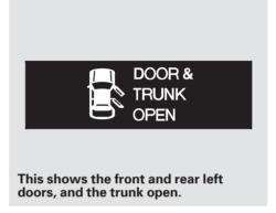
When one or more doors and the trunk lid are not tightly closed, the corresponding indicator for each condition and the "DOOR & TRUNK OPEN" indicator will come on.
