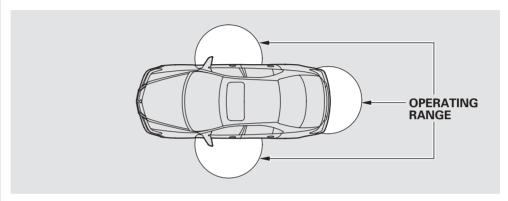
You can lock/unlock the doors within about a 32 inch (about 80 cm) radius from the outside door handle. You can open the trunk within about a 32 inch (about 80 cm) radius from the trunk release switch.
