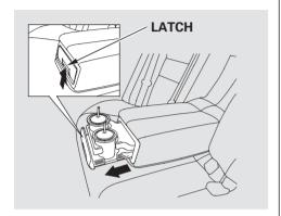
The rear beverage holder is in the rear seat armrest. Open the beverage holder by pulling up on the latch on the front.
