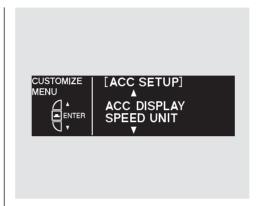
While the multi-information display is in the ACC SETUP of the CUSTOMIZE GROUP, press the SEL/RESET button. The screen changes to CUSTOMIZE MENU. Press the INFO (▲/▼) button until you see the above display.
