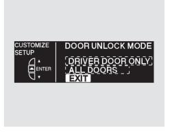
To exit DOOR UNLOCK MODE without changing the current setting, select EXIT by pressing the INFO (▲/▼) button, then press the SEL/RESET button. The screen goes back to CUSTOMIZE MENU.
