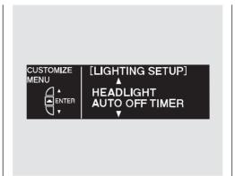
While the multi-information display is in the LIGHTING SETUP screen of the CUSTOMIZE GROUP, press the SEL/RESET button. The screen changes to CUSTOMIZE MENU. Press the INFO (▲/▼) button until you see the above display.
