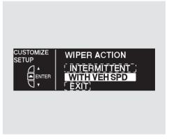
Press the SEL/RESET button. The screen changes as shown above. Select INTERMITTENT or WITH VEH SPD by pressing the INFO (▲/▼) button, then press the SEL/RESET button to enter your selection.
