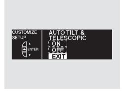
To exit AUTO TILT & TELESCOPIC without changing the current setting, select EXIT by pressing the INFO (▲/▼) button, then press the SEL/RESET button. The screen goes back to CUSTOMIZE MENU.
