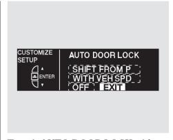
To exit AUTO DOOR LOCK without changing the current setting, select EXIT by pressing the INFO (▲/▼) button, then press the SEL/RESET button. The screen goes back to CUSTOMIZE MENU.
