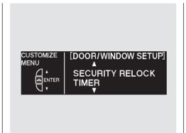
While the multi-information display is in the DOOR/WINDOW SETUP screen of the CUSTOMIZE GROUP, press the SEL/RESET button. The screen changes to CUSTOMIZE MENU. Press the INFO (▲/▼) button until you see the above display.
