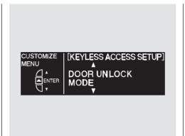
While the multi-information display is in the KEYLESS ACCESS SETUP screen of the CUSTOMIZE GROUP, press the SEL/RESET button. The screen changes to the above display.
