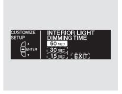
Press the SEL/RESET button. The screen changes as shown above. Select how long you want the lights to stay on before they fade out (60, 30, or 15 seconds) by pressing the INFO (▲/▼) button, then press the SEL/RESET button to enter your selection.
