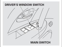
Turn the ignition switch to the ON (II) position before operating any of the window switches. To open a window, push the switch down and hold it. To close the window, pull the switch up and hold it. Release the switch to stop the window.
