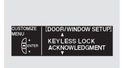
While the multi-information display is in the DOOR/WINDOW SETUP screen of the CUSTOMIZE GROUP, press the SEL/RESET button. The screen changes to CUSTOMIZE MENU. Press the INFO (▲/▼) button until you see the above display.
