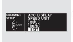
To exit ACC DISPLAY SPEED UNIT without changing the current setting, select EXIT by pressing the INFO (▲/▼) button, then press the SEL/RESET button. The screen goes back to CUSTOMIZE MENU.
