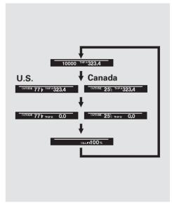
With the ignition switch in the ON (II) position, the lower part of the multi-information display changes as shown in the illustration, each time you press the SEL/RESET button.
