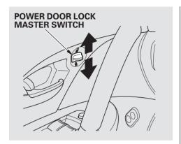
Each front door has a power door lock master switch. Either switch locks and unlocks all doors. Push the switch down to lock all doors and up to unlock them.
