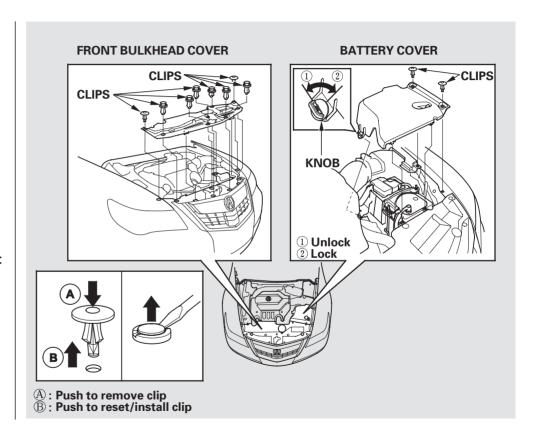
To remove the left engine compartment cover:
