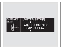
While the multi-information display is in the METER SETUP of the CUSTOMIZE GROUP, press the SEL/RESET button. The screen changes to CUSTOMIZE MENU. Press the INFO (▲/▼) button until you see the above display.
