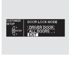
To exit DOOR LOCK MODE without changing the current setting, select EXIT by pressing the INFO (▲/▼) button, and then press the SEL/RESET button. The screen goes back to CUSTOMIZE MENU.
