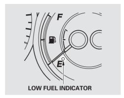
This indicator is in the fuel gauge. It comes on as a reminder that you must refuel soon. You will also see a "FUEL LOW" message on the multi-information display. When the indicator comes on, there are about 2.69 U.S. gal  $(10.2 \ \ell)$  of fuel remaining in the tank. When the needle reaches E, there is a very small amount of fuel in the tank
