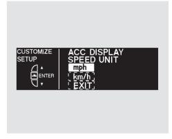
Press the SEL/RESET button. The screen changes as shown above. The highlighted unit, mph or km/h, is the current setting. To change the setting, press the INFO  $(\triangle/\nabla)$  button until the unit you want is highlighted, then press the SEL/RESET button.
