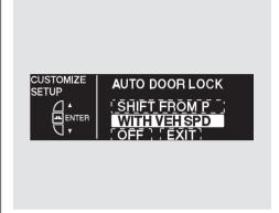
Press the SEL/RESET button. The screen changes as shown above. Select the desired setting by pressing the INFO (▲/▼) button, then press the SEL/RESET button to enter your selection.
