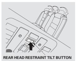
3. Turn the ignition switch to the ON (II) position, then push the rear head restraint tilt button on the ceiling console to pivot the head restraints down.
