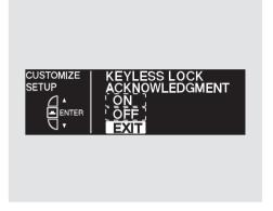
To exit KEYLESS LOCK ACKNOWLEDGMENT without changing the current setting, select EXIT by pressing the INFO (▲/▼) button, then press the SEL/RESET button. The screen goes back to CUSTOMIZE MENU.
