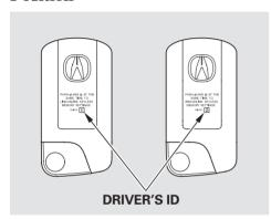
When you unlock the driver's door with your remote transmitter, each remote transmitter activates the customized settings related to that remote.
