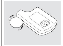
Replace the batteries if necessary. Battery type: CR2025
