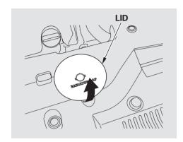
1. Lift up the lid on the front bulkhead cover from the front.
