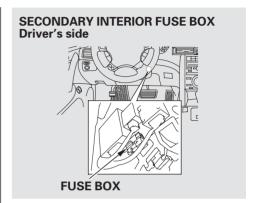
To open the secondary fuse box lid, push the tab in the direction as shown in the illustration.
