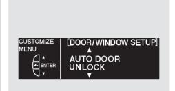
While DOOR/WINDOW SETUP is shown in the CUSTOMIZE GROUP of the multi-information display, press the SEL/RESET button. The screen changes to CUSTOMIZE MENU. Press the INFO (▲/▼) button until you see the above display.
