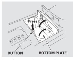
For a long container, press the button in the beverage holder to raise the bottom plate. Stand the separator up.
