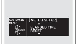
While METER SETUP is shown in the CUSTOMIZE GROUP of the multi-information display, press the SEL/RESET button. The screen changes to CUSTOMIZE MENU. Press the INFO (▲/▼) button until you see the above display.
