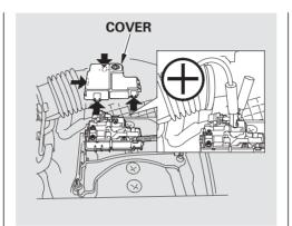
3. Remove the battery cover (see page 492), then remove the secondary under-hood fuse box cover from the positive (+) terminal on the battery.
