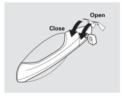
You can open and close the windows and moonroof with the built-in key in the driver's door lock.
