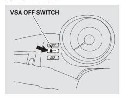
This switch is at the right side of the left vent. To turn the VSA system on and off, press and hold it until you hear a beep.
