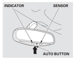
The inside mirror can automatically darken to reduce glare. To turn on this feature, press the button on the bottom of the mirror. The AUTO indicator comes on as a reminder. When it is on, the mirror darkens when it senses the headlights of a vehicle behind you, then returns to normal visibility when the lights are
