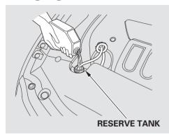
If the coolant level in the reserve tank is at or below the MIN line, add coolant to bring it up to the MAX line. Inspect the cooling system for leaks. Always use Honda Long-life Antifreeze/Coolant Type 2. This coolant is pre-mixed with 50 percent antifreeze and 50 percent distilled water. Never add straight antifreeze or plain water.
