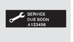
When the engine oil life reaches 15%, the display shows "SERVICE DUE SOON" and the code for the maintenance items to be performed.
