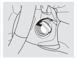
When you push the ignition switch, the remote and the vehicle recognize each other. After the recognition, the remote indicator flashes, and a beeper sounds once. After the beep, turn the ignition switch.
