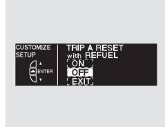
Press the SEL/RESET button. The screen changes as shown above. Select ON or OFF by pressing the INFO (▲/▼) button, then press the SEL/RESET button to enter your selection.
