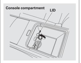
The other socket is under the armrest in the console compartment storage area. To use the power socket, pull up the cover.
