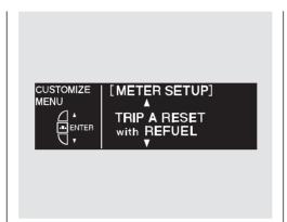
While METER SETUP is shown in the CUSTOMIZE GROUP of the multi-information display, press the SEL/RESET button. The screen changes to CUSTOMIZE MENU. Press the INFO (▲/▼) button until you see the above display.
