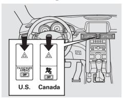
Push the button between the center vents to turn on the hazard warning lights (four-way flashers). This causes all four outside turn signals and both indicators in the instrument panel to flash. Use the hazard warning lights if you need to park in a dangerous area near heavy traffic, or if your vehicle is disabled.
