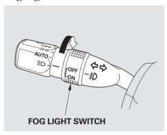
Turn the fog lights on and off by turning the switch next to the headlight switch.
