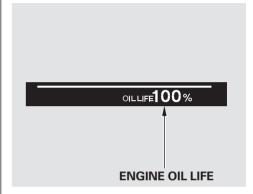
This shows the remaining life of the engine oil. It shows 100% after the engine oil is replaced and the display is reset. The engine oil life is calculated based on engine operating conditions and accumulated engine revolutions. For more information, see page 445.
