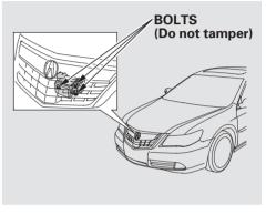
There are three bolts on the sides of the radar sensor. Do not tamper with these bolts, or you may cause the system to malfunction.
