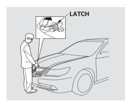
2. Reach between the hood and the front bumper with your finger. Slide the latch handle up.
