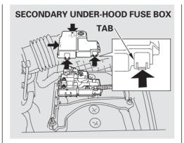
The secondary under-hood fuse box is on the battery. To open it, push the tabs as shown.
