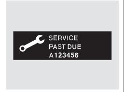
If the indicated maintenance service is not done and the remaining engine oil life reaches 0%, the multi-information display will show the message "SERVICE PAST DUE" and the maintenance item code(s). This message is displayed when the total distance traveled is less than 10 miles (for U.S. models) or 10 km (for Canadian models) after the engine oil life became 0%.
