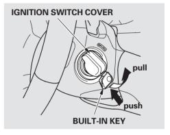
To remove the ignition switch cover, insert the built-in key (see page 181), then pull the cover out by pulling the built-in key while pushing it.
