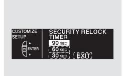
Press the SEL/RESET button. The screen changes as shown above. Select the relock time you want (90, 60, or 30 seconds) by pressing the INFO (▲/▼) button, then press the SEL/RESET button to enter your selection.
