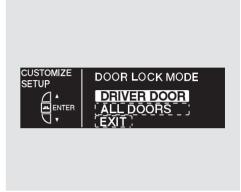
Press the SEL/RESET button. The screen changes as shown above. Select DRIVER DOOR or ALL DOORS by pressing the INFO (▲/▼) button, then press the SEL/RESET button to enter your selection.
