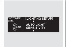
While LIGHTING SETUP is shown in the CUSTOMIZE GROUP of the multi-information display, press the SEL/RESET button. The screen changes to CUSTOMIZE MENU. Press the INFO (▲/▼) button until you see the above display.
