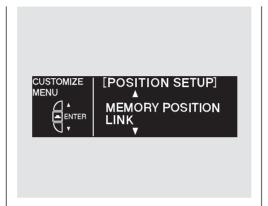
While the multi-information display is in the POSITION SETUP screen of the CUSTOMIZE GROUP, press the SEL/RESET button. The screen changes to the above display.
