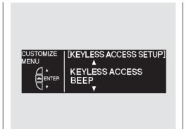
While the multi-information display is in the KEYLESS ACCESS SETUP screen of the CUSTOMIZE GROUP, press the SEL/RESET button. The screen changes to CUSTOMIZE MENU. Press the INFO (▲/▼) button until you see the above display.
