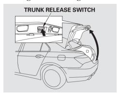
When the trunk is locked, you can open it in any of these ways:
