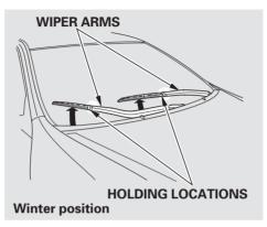
Adjust the wiper arms to the winter position by holding both arms as shown in the illustration at the same time. Pull on the arm, parallel to the windshield, until it locks in the higher position.
