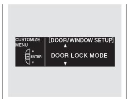
While the multi-information display is in the DOOR/WINDOW SETUP screen of the CUSTOMIZE GROUP, press the SEL/RESET button. The screen changes to CUSTOMIZE MENU. Press the INFO (▲/▼) button until you see above display.
