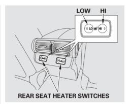
The ignition switch must be in the ON (II) position to use seat heaters. Push the right side of the switch, HI, to rapidly heat up the seat. After the seat reaches a comfortable temperature, select LO by pushing the left side of the switch. This will keep the seat warm.
