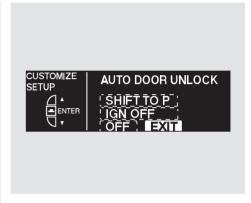
To exit AUTO DOOR UNLOCK without changing the current setting, select EXIT by pressing the INFO (▲/▼) button, then press the SEL/RESET button. The screen goes back to CUSTOMIZE MENU.
