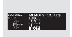
To exit MEMORY POSITION LINK without changing the current setting, select EXIT by pressing the INFO (△/▼) button, then press the SEL/RESET button. The screen goes back to CUSTOMIZE MENU.
