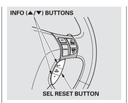
You can change the display and customize your vehicle control settings by pressing the SEL/RESET or INFO buttons on the right side of the steering wheel.
