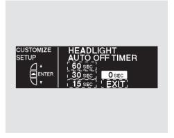
Press the SEL/RESET button. The screen changes as shown above. Select how long you want the lights to stay on before they go off (0, 15, 30, or 60 seconds) by pressing the INFO  $(\triangle/\nabla)$  button, then press the SEL/RESET button to enter your selection.
