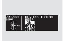
Press the SEL/RESET button. The screen changes as shown above. Select ON or OFF by pressing the INFO (▲/▼) button, then press the SEL/RESET button to enter your selection.
