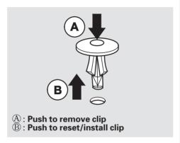
2. Remove the holding clips by pushing on the center of each fastener head.
