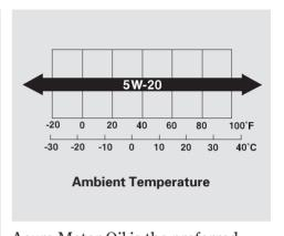
Acura Motor Oil is the preferred 5W-20 lubricant for your vehicle. It is highly recommended that you use Acura Motor Oil in your vehicle for optimum engine protection. Make sure the API Certification Seal says "For Gasoline Engines." The oil viscosity or weight is provided on the container's label. 5W-20 oil is formulated for yearround protection of your vehicle to improve cold weather starting and fuel economy.
