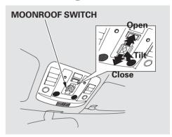
Turn the ignition switch to the ON (II) position before operating the moonroof switch on the ceiling console. To open the moonroof, pull back the moonroof switch. To close the moonroof, push the moonroof switch forward. Release the switch to stop the moonroof.
