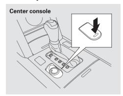
There are two accessory power sockets. One is located in the front of the center console. To use the power socket, push and release the lid.
