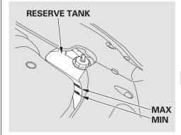
Look at the coolant level in the radiator reserve tank. Make sure it is between the MAX and MIN lines. If it is below the MIN line, see **Adding Engine Coolant** on page 461 for information on adding the proper coolant.
