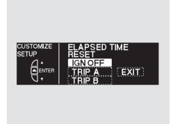
Press the SEL/RESET button. The screen changes as shown above. Select the desired setting by pressing the INFO (▲/▼) button, then press the SEL/RESET button to enter your selection.
