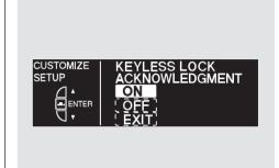
Press the SEL/RESET button. The screen changes as shown above. Select ON or OFF by pressing the INFO (▲/▼) button, then press the SEL/RESET button to enter your selection.
