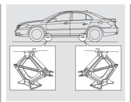
7. Place the jack under the jacking point nearest the tire you need to change. It is pointed to by a △ mark molded into the underside of the body. Turn the end bracket clockwise until the top of the jack contacts the jacking point. Make sure the jacking point tab is resting in the jack notch.
