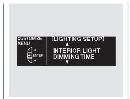
While LIGHTING SETUP is shown in the CUSTOMIZE GROUP of the multi-information display, press the SEL/RESET button. You will see the above display.
