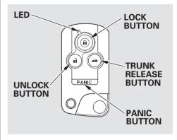
LOCK — Press this button once to lock all doors. Some exterior lights will flash. When you push the LOCK button twice within 5 seconds, you will hear a beep to verify that the doors are locked and the security system is set.
