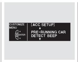
While the multi-information display is in the ACC SETUP of the CUSTOMIZE GROUP, press the SEL/RESET button. The screen changes to the above display.
