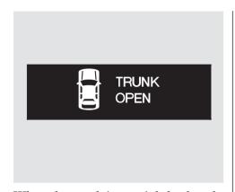
When the trunk is not tightly closed, the "TRUNK OPEN" indicator will come on.
