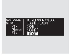
To exit KEYLESS ACCESS LIGHT FLASH without changing the current setting, select EXIT by pressing the INFO (▲/▼) button, then press the SEL/RESET button. The screen goes back to CUSTOMIZE MENU.
